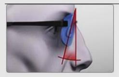
This is the angle in the vertical plane between the optical axis of a spectacle lens and the visual axis of the eye in primary position.
