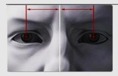
This is the distance from the axis of symmetry of the face (the centre of the nose) to the centre of the pupil. It is recommended to measure the naso-pupillary distance for each eye separately.
