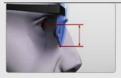
This is the vertical distance from the pupil centre to the bottom of the frame when the wearer is looking straight ahead. It is recommended to measure it for each eye separately.
